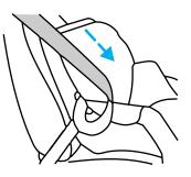
6. Allow the belt to retract. The belt will click as it retracts to indicate it is in the automatic locking mode.
